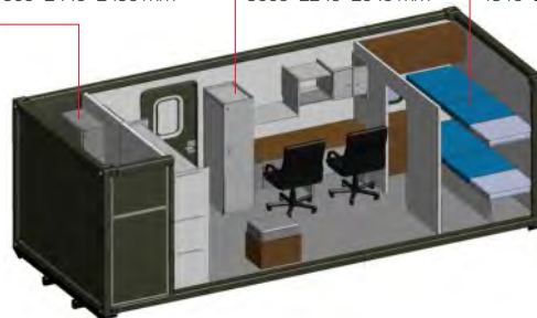
Service module 960×2440×2490 mm Working area 3660×2240×2040 mm Living area 1310×2240×2040 mm
