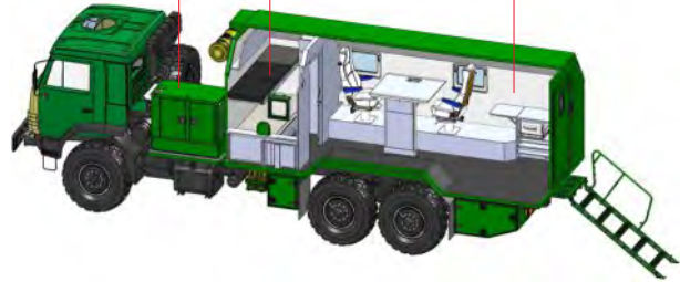
Service module 1400×2450×1520-2150 mm Living area 1330×2350×2050 mm Working area 4500×2350×2050 mm
